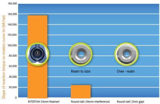
Compared to traditional cylindrical designs, it takes more torque to cause a TRIGEN INTERTAN nail's proximal section to rotate in the proximal femur.
